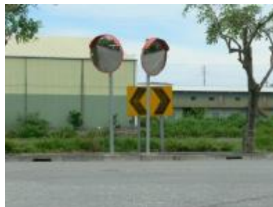
After starting Dong-Cheng Safe Community Program in January 2006, the Road traffic mirror was installed on the main three-forked road before entering the community for preventing car accidents.
